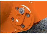
The bucket hinge pins are hermetically sealed to retain grease inside for longer service life.
