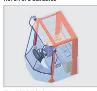
This ROPS/FOPS cab is adopted to protect the operator from injury in the case of an accident. ROPS: Roll-Over Protective Structure,
