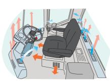
The air conditioner/heater is controlled automatically and thermostatically to enhance operator comfort. Air vents promote good air circulation inside, and defrosting all the year around. The cab is pressurized to keep out dirt.
