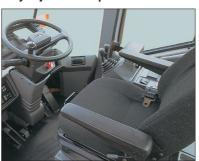
The suspension seat is fully adjustable for riding comfort, reducing operator fatigue and increasing operator's productivity.
