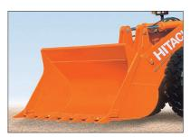
The strong lift arms and linkage yield high production during digging, loading and hauling. Big bucket breakout force and optimum bucket rollback bring about high production and good load retention. Buckets are designed and shaped for efficient scooping-up and loading. Bolton cutting edges are easy to replace. The bucket leveler and boom kickout come standard.
