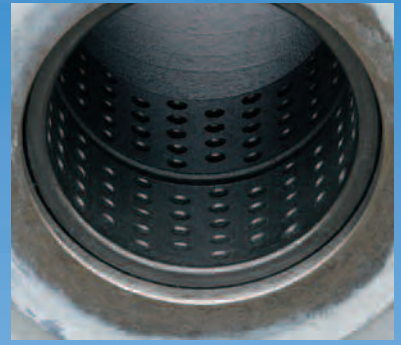
Flanged brass bushings provide long life and extended maintenance intervals.
