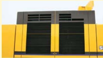
Bolted double service doors
