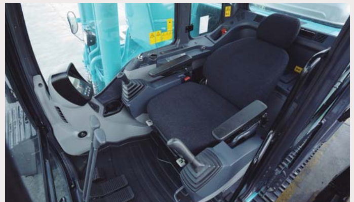
● Seat can be reclined to horizontal position
