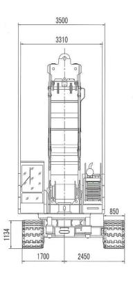
Main Dimensions for SCC800C Hydraulic Crawler Crane
