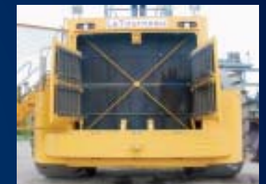
Typical of LeTourneau 50 Series serviceability, the hinged grill and braking grids swing out of the way for easy radiator access.
