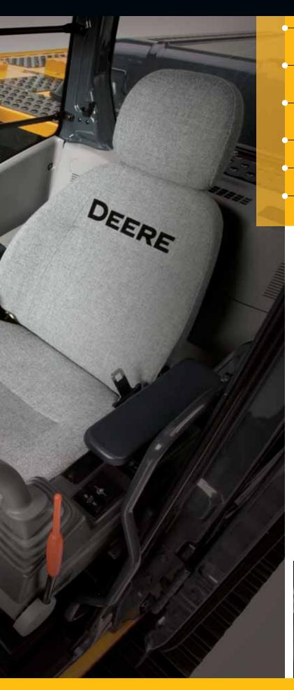
Deluxe-suspension multi-position seat has 10½ inches of travel, sliding together or independent of the control console. So it won't cramp an operator's style.
