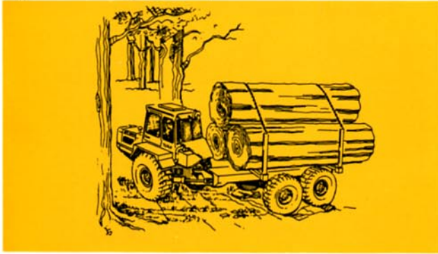
TC 860 for heavy log hauling with bunks, stakes and winch.
