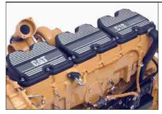
**Diesel Engine.** The Caterpillar C18, with ACERT technology, is a 18.1 liter, six-cylinder, 390 kW (530 hp) engine with mechanically actuated electronic fuel injection (MEUI) and overhead camshaft. ACERT technology provides outstanding engine performance through advanced electronic control, precision fuel delivery, and refined air management.
