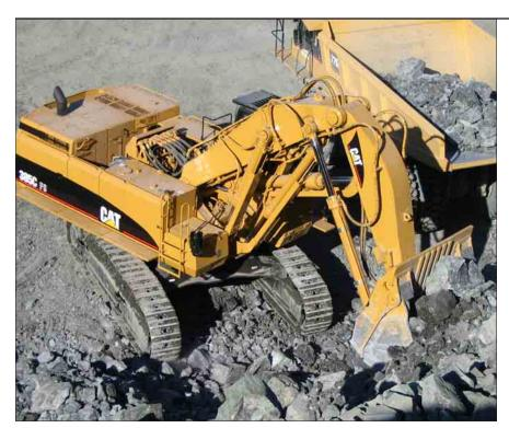
Hydraulic System. The 385C FS hydraulic system includes a three-pump system with an independent swing circuit and a hydraulic circuit utilizing the proven Proportional Priority Pressure Compensated (PPPC) system. It features Caterpillar-developed electronic control and activation to ensure high hydraulic system efficiency and excellent productivity.
