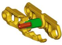
**Track.** The 385C comes standard with the new grease lubricated track called GLT4. The track links are assembled and sealed with grease to decrease internal bushing wear, reduce travel noise and extend service life lowering operating costs.
