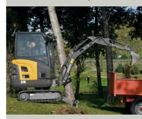
Protected, smartly-positioned boom cylinder.
