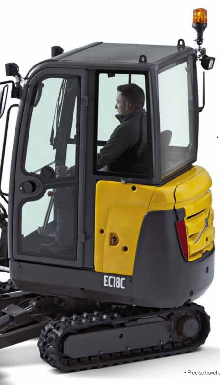
• Operate in a protected TOPS/ROPS/OPG1 safety structure.
