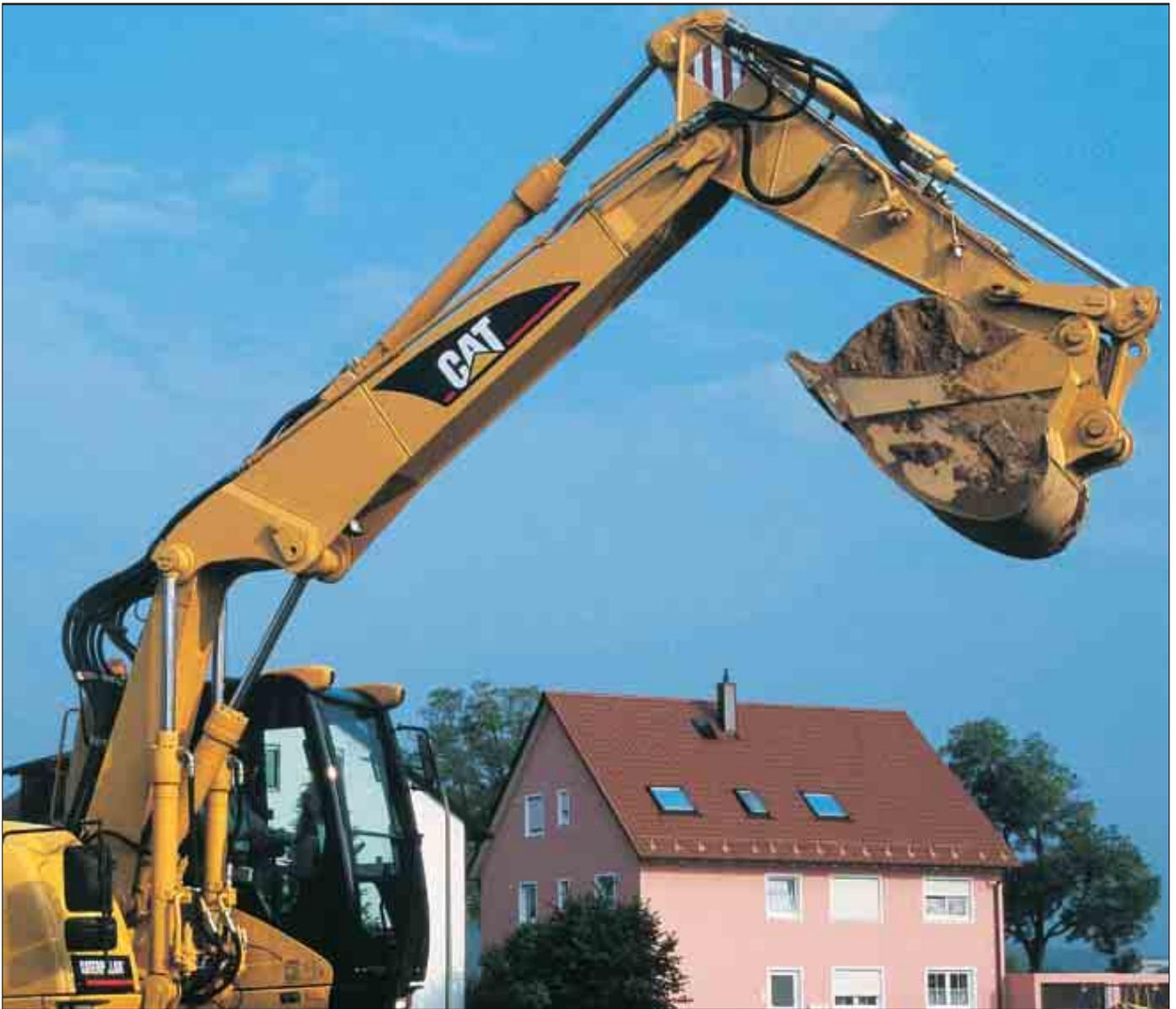
**Booms and Sticks.** Built for performance and long service life, Caterpillar booms and sticks are large, welded, box-section structures with thick, multi-plate fabrications in high-stress areas.
