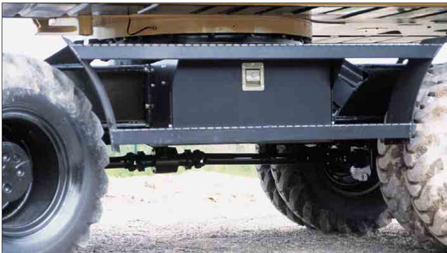
**Tool Box.** A large sealed and lockable toolbox is mounted on the undercarriage between the steps on the machine's left side. A second optional toolbox is available for the right side.
