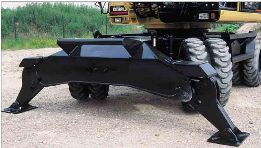
**Outriggers.** Recommended for maximum operating stability when digging and lifting, the outriggers can be individually controlled to level the machine on slopes. Featuring pin-on design, heavy-duty cylinder guards, and optimized kinematics, the outriggers can be mounted on the front, rear or on both ends of the machine.
