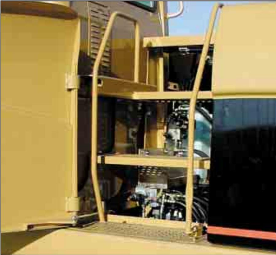
**Extended Service Intervals.** M313C service and maintenance intervals have been extended to reduce machine service time, increase machine availability and reduce operating costs. Using S•O•S hydraulic oil change intervals can be extended from 2000 hours to 4000 hours. Engine coolant change intervals are up to 6000 hours when Cat Extended Life Coolant/Anti-Freeze is used.
