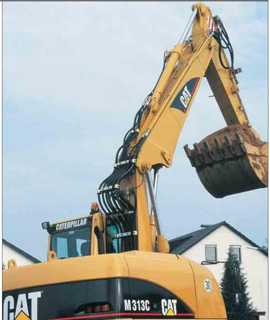
**Hydraulic Cylinder Snubbers.** The hydraulic cylinder snubbers at the rod end of boom cylinders, both ends of stick cylinders, and bucket cylinder rod end cushion shocks, reduce sound and increase cylinder life, keeping the machine working longer.
