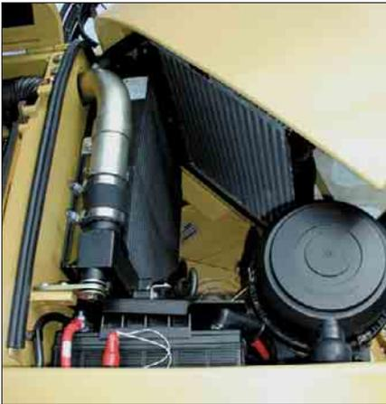
**Powerful Performance.** The 3054E ATAAC engine delivers a net power of 86 kW (115 hp) at the rated speed of 2000 rpm, and meets all current worldwide emission standards.
