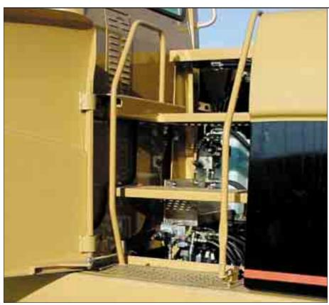
Extended Service Intervals. M316C service and maintenance intervals have been extended to reduce machine service time, increase machine availability and reduce operating costs. Using S•O•S hydraulic oil change intervals can be extended from 2000 hours to 4000 hours. Engine coolant change intervals are up to 6000 hours when Cat Extended Life Coolant/Anti-Freeze is used.
