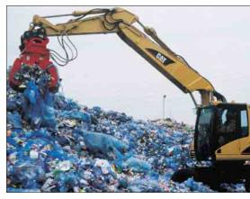
**Demolition and Sorting Grapple.** The demolition and sorting grapple with unlimited left and right rotation is the ideal tool for stripping, sorting, handling and loading.
