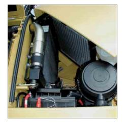
**Powerful Performance.** The 3056E ATAAC engine delivers a net power of 113 kW (151 hp) at the rated speed of 2000 rpm, and meets all current worldwide emission standards.
