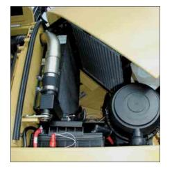
**Powerful Performance.** The 3056E ATAAC engine delivers a net power of 122 kW (164 hp) at the rated speed of 2000 rpm, and meets all current worldwide emission standards.
