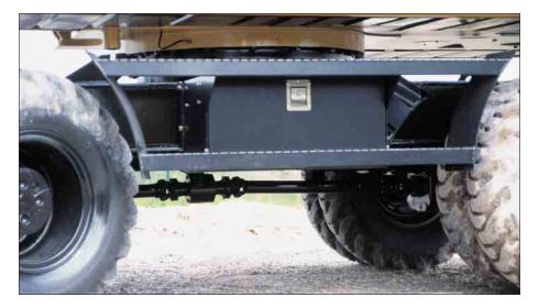
A Strong Undercarriage. The welded frame provides excellent rigidity and long life. Efficient hydraulic lines routing, transmission protection and heavy-duty axles make the undercarriage perfect for wheel excavator applications. Both outriggers and dozer blade are pin-on for maximum flexibility.
