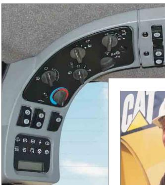
**Controls.** The main control panel on the 980H is located high on the right ROPS post – keeping everything within reach of the operator while maintaining visibility to the ground. Keeping all switches and controls conveniently placed allows better operator efficiency and improved productivity, while minimizing operator fatigue.
