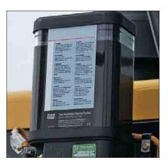
Autolube. Reduce time spent on daily maintenance and downtime for unplanned repairs due to inadequate greasing with the optional Caterpillar Automatic Lubrication System. Precise lubrication of pins and bushings at specific intervals decreases component wear and reduces ground contamination from excessive greasing.
