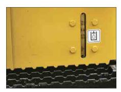
**Sight Gauges.** Well-protected, yet easily visible sight gauges for the transmission oil, hydraulic oil and engine coolant allow easy daily checks while reducing the risk of contaminants entering the systems.
