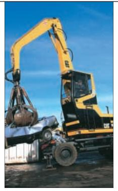
**The fixed cab riser** offers a very stable and comfortable method to raise the cab. The fixed cab riser lifts the cab by 1.2 m to offer better viewing to all sides. In shipping position, the cab is unmounted to meet national road regulations.
