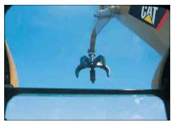
**Viewing Area.** To maximize visibility, all glass is affixed directly to the cab, eliminating the use of window frames. Choice of fixed or easy-to-open split front windshields meet operator preference and application conditions.
