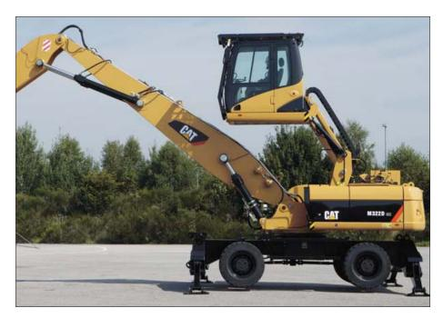
**Top Position**. The top position raises the cab by 2400 mm. This provides optimal viewing for all material handling jobs.
