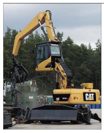
**MH Booms and Sticks.** The MH booms have been redesigned to handle increased lifting capacities. The new stick range offers leading side plates to maximize the protection of hydraulic lines. The lines are fitted in between the two side plates offering protection from damage. Multiple boom and stick options allow you to pick the best match for your job.
