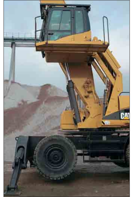
Top Position. The top position raises the cab by 2600 mm. This provides optimal viewing to all sides in different applications such as scrap handling and port handling. The cab can be positioned at any level between lowest and highest positions.
