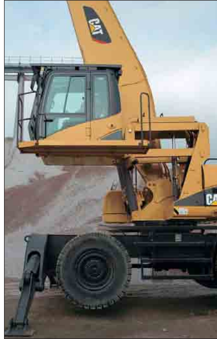
Medium Position. The medium position places the cab forward by 500 mm more than in the travel position, for increased visibility.
