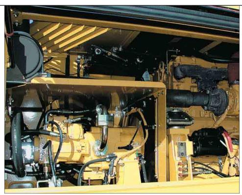
Ground Level Service. The design and layout of the M313C was made with the service technician in mind. The fuel water separator, engine oil filter, battery, radiator fluid level, fuel filter, engine oil gauge, hydraulic oil level, air cleaner and pilot system filter are all easily accessible at ground level allowing critical maintenance to be done quickly and efficiently.
