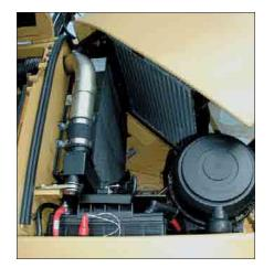
**Powerful Performance.** The 3054E DIT ATAAC engine delivers a net power of 88 kW (120 hp) at the rated speed of 2000 rpm, and meets all current worldwide emission standards.
