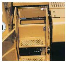
**Extended Service Intervals.** M313C service and maintenance intervals have been extended to reduce machine service time, increase machine availability and reduce operating costs. Using S•O•S hydraulic oil change intervals can be extended from 2000 hours to 4000 hours. Engine coolant change intervals are up to 12 000 hours with using Cat Extended Life Coolant/Anti-Freeze.
