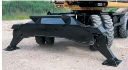
**Outriggers.** The pin-on design allows the outriggers to be mounted on the front and/or rear for maximum operating stability when digging or lifting and are individually controlled for leveling on slopes.
