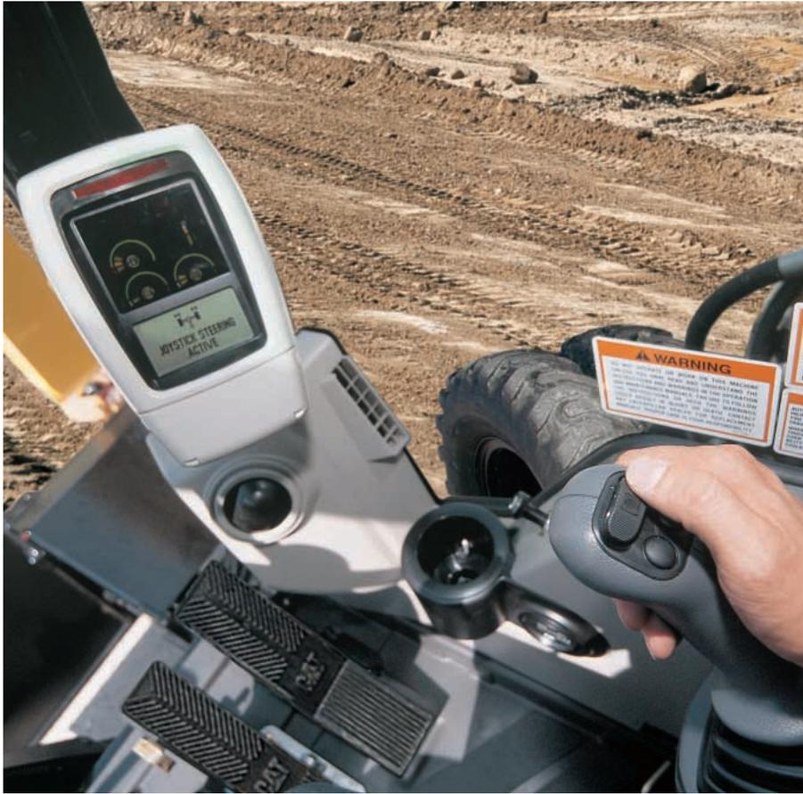
**Joystick Steering.** Enables an operator to steer the machine in the first gear while simultaneously working the implements, keeping both hands on the joysticks. The operator is more productive using this feature.
