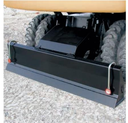
**Dozer Blade.** The pin-on design allows the dozer blade to be mounted on the front and/or rear and is used for leveling, clean-up work and for stabilizing the machine during digging applications. The large dozer bottom and parallel design provide minimized ground pressure.
