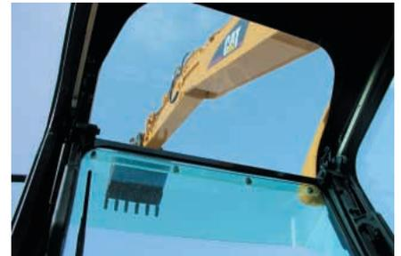
**Skylight.** A unique large polycarbonate skylight provides excellent upward visibility.
