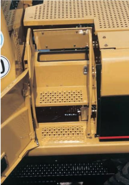
**Handrails and Steps.** Large handrails and steps assist the operator in climbing on and off the machine.
