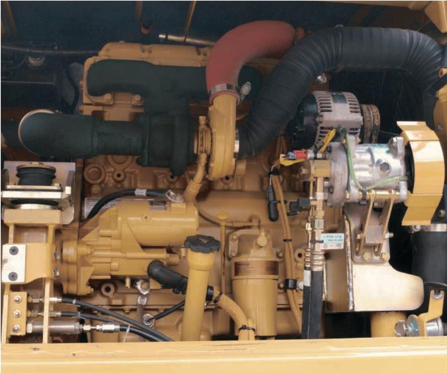
**Powerful Performance.** The 3054E DIT ATAAC engine delivers a net power of 91 kW (121 hp) at the rated speed of 2,000 rpm, and meets U.S. EPA Tier 2 emission standards.
