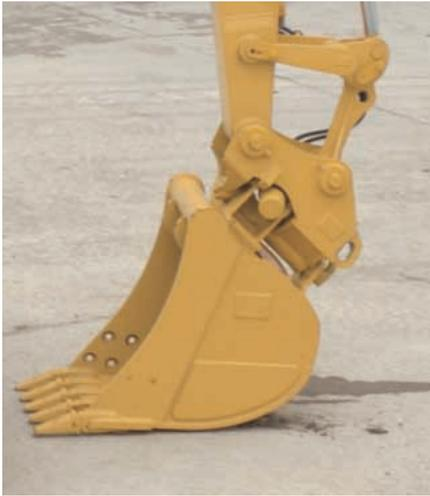
**Buckets.** Caterpillar offers five general purpose buckets, one extreme service bucket and three ditch cleaning buckets.
