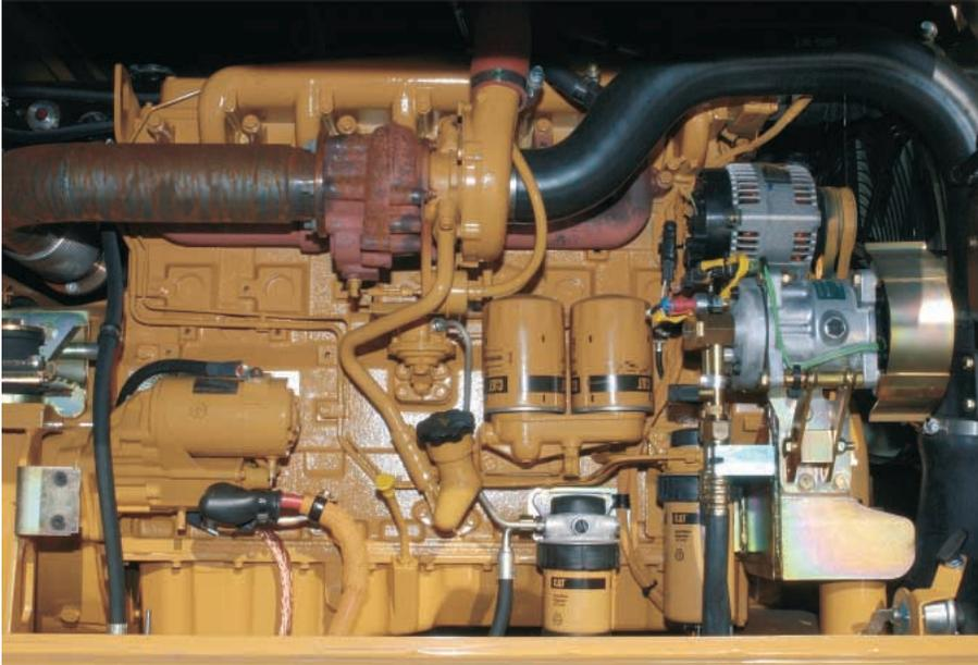
**Powerful Performance.** The 3056E DIT ATAAC engine delivers a net power of 103 kW (138 hp) at the rated speed of 2,000 rpm, and meets U.S. EPA Tier 2 emission standards.
