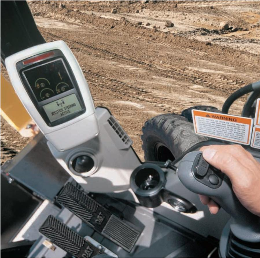
**Joystick Steering.** Enables an operator to reposition the machine in the first gear while simultaneously working with the implements, keeping both hands on the joysticks. The operator is more productive using this feature.
