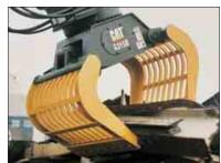
**Multi-Processor.** The Caterpillar Multi-Processors can be equipped with different jaw types depending on your need.
