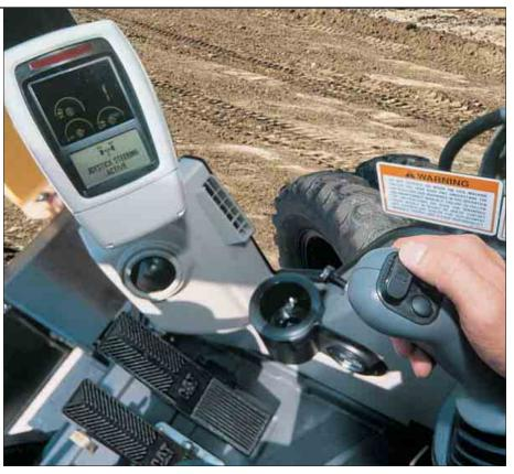
**Power Modes.** There are three power mode settings. The operator can choose the best power setting for both engine and hydraulic power versus fuel efficiency.
