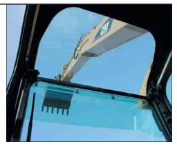
**Skylight.** A unique large polycarbonate skylight provides excellent upward visibility.
