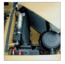
**Powerful Performance.** The 3056E DIT ATAAC engine delivers a net power of 122 kW (164 hp) at the rated speed of 2000 rpm, and meets all current worldwide emission standards.
