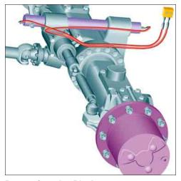
Remote Greasing Block. A greasing block is located in the engine compartment on the upper carriage, with two grease points for the swing bearing and one for the front end attachment. This delivers grease to hard-to-reach locations. For the lower undercarriage, two remote blocks give easy access for greasing to the oscillating axle and, as an option, the dozer blade.
