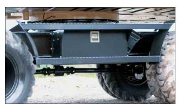
**Strong Undercarriage.** The welded frame provides excellent rigidity and long life. Efficient hydraulic lines routing, transmission protection and heavy-duty axles make the undercarriage perfect for wheel excavator applications. Both outriggers and dozer blade are pin-on for maximum flexibility.
