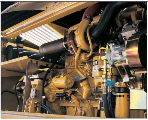
Ground Level Service. The design and layout of the M322C was made with the service technician in mind. The fuel water separator, engine oil filter, battery, radiator fluid level, fuel filter, engine oil gauge, hydraulic oil level, air cleaner and pilot system filter are all easily accessible at ground level allowing critical maintenance to be done quickly and efficiently.
