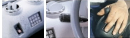
Left: Ten air outlets provide fresh filtered and climate-controlled air. Contrinsic II control panel allows direct access to all major monitoring functions.
