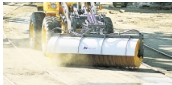
Thanks to the hydrostatic transmission, with its inching function**, the L50D can maximise power to the attachments while operating at very low speeds.
