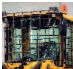
Windshield guard Protects both the cab glass and operator from debris. It is custom designed to minimize glass breakage while maximizing visibility. (L60E–L220E)
