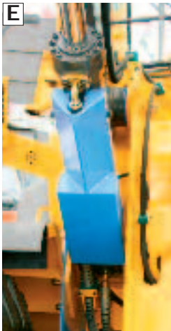
E Boom cylinder hose and tube guards Designed to protect the boom cylinder hoses and tubes, these “box-type” structures prevent debris from breaking the hoses and/or tubes when debris becomes trapped between the front frame and the boom cylinders. Steel spiral hose guards and a protective plate are used to cover the hoses connecting the boom cylinders to the main valve. (L60E–L220E)
