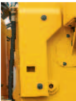
Grease tube guards Protective guarding is used to cover exposed grease tubes and zerks. (L70E–L220E)
