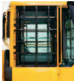
Window guards, side and rear Provide protection for both the side and rear windows. The two side window guards are hinged for easy cleaning and maintenance, while the rear window guard can easily be removed by means of two quickdisconnect latches. (L60E–L220E)
