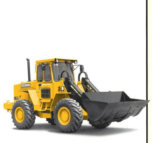
ENGINE OUTPUT: 110 hp (81 kW) VOLVO DIRECT-INJECTED, TURBO-CHARGED DIESEL
