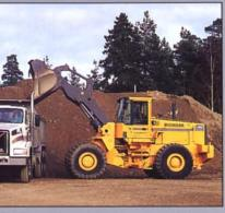
High positioned loader arms with a long reach facilitate loading onto high-sided vehicles. The adjustable, boom and bucket kick out mechanism automatically assumes the proper position for a level bucket and the optimum height for dumping.
