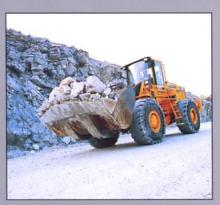
Fully floated axles. The front axle with 100% differential lock, including sealed wet and cooled disc brakes provide a high degree of safety and long life.
