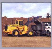
Torque Parallel linkage gives both high breakout torque and parallel action within the whole lifting range. High, controlled tilt speeds contribute to short cycle times and a minimum of spillage.
