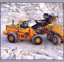
The new loader unit Torque Parallel linkage is designed for demanding production work such as quarrying. Torque Parallel linkage brings together the best from Michigan parallel-system with advantages from the traditional Z-bar linkage.
