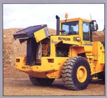
Large, gas strutted hatches for the engine compartment facilitate service and inspection. The large radiator hood and the swing-out radiator give easy access to the radiator from all sides for cleaning.
