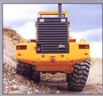
The rear axle can oscillate 15° without shifting the machine's center of gravity. This rear axle oscillation also means that all the wheels remain in contact with the ground even when operating in uneven terrain.
