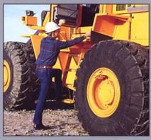
A wide door with a wide opening angle and slip-free ladder with 15 degree incline make entering and leaving the cab effortless. Well-positioned handles and footsteps on both sides of the machine facilitate inspection and maintenance.
