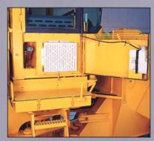
The efficient climate control system with replaceable air filters, gives you the ideal working temperature in all possible conditions. A total of 14 adjustable vents, including a 4-speed fan, circulates dust-free air evenly throughout the cab.
