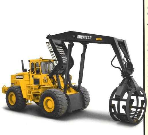
ENGINE OUTPUT: 252 hp (185 kW) VOLVO DIRECT-INJECTED, TURBOCHARGED DIESEL
