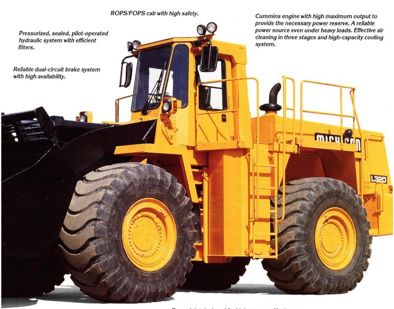
Large planetary-type hub reductions greatly reduce the stresses on the drivetrain components. Low-friction roller bearings reduce heat buildup.
