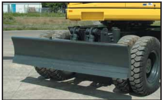
Dozer blade A parallel blade is available with standard cylinders protector for both the front and rear of the machine. Dimensions: 2.550 mm x 520 mm
