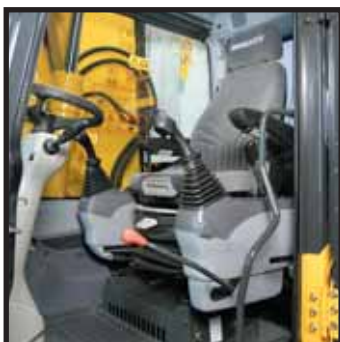
Seat sliding range: 340 mm
