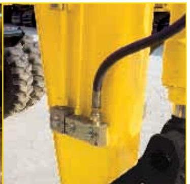
■ INTEGRIERTES UMSCHALTVENTIL
