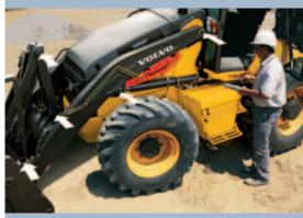
50-hour greasing intervals, and all greasing points are accessible from the ground level.
