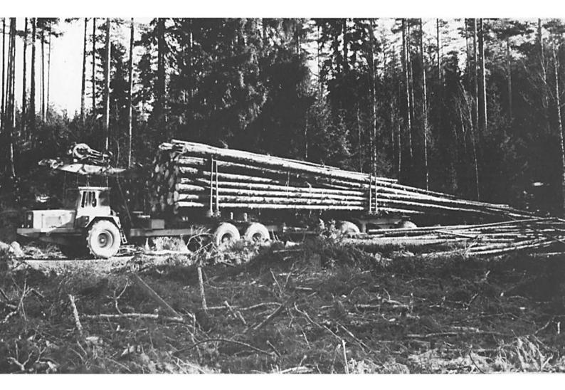
VOLVO BM 860 TC tree length hauler. Trailer with turntable ensures agile manoeuvrability. Accommodates logs up to 30 m in length.
