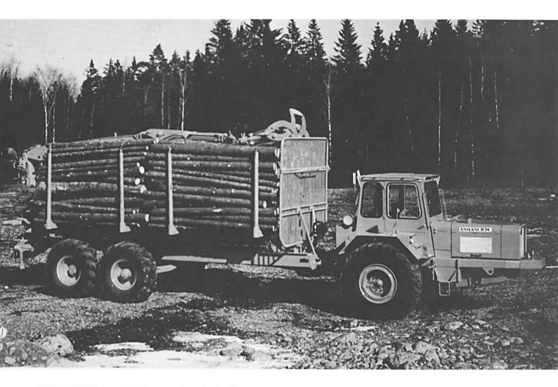
VOLVO BM 860 TC forwarder, long version, for hauling shortwood. Carries two stacks of 3-m pulpwood or logs up to 7 m in length.
