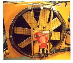
The fan is driven by a thermostatically controlled hydraulic motor. This continuously regulates the fan speed, drawing power only when needed.
