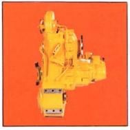
The drop-box has a built-in differential with a lock-up function. Power take-off from the drop-box also drives the safety steering pump. This guarantees full steering capacity as soon as the machine is rolling.
