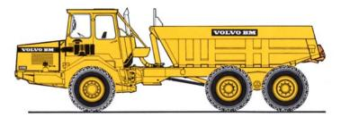
**Basic body** with wear plates for forced loading of rubble or similar material. This body is prepared with ducts for exhaust gas heating.
