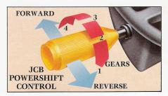
• JCB Powershift transmission pravides fast gear changing without losing speed on gradients. A column-mounted, light electrictwist grip allows the operator to control machine direction and change gear effortlessly.
