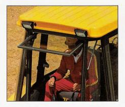
• Gas strut assisted rear window which slides into roof but projects slightly to provide rain protection for the operator.
