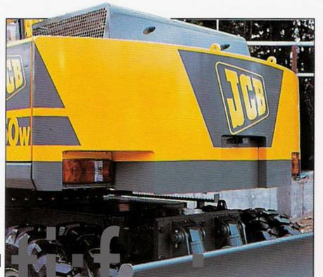
hydraulic system. The selectable work modes match the hydraulic output to the requirements of the job for maximum operating efficiency.
