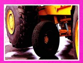
Volvo BM has developed a completely new turnaround system specially for the  $5350 \text{ B} 4\times4$ . This consists of a wheelequipped bridge that is operated hydraulically from the cab. The operator can simply rotate the trailer unit a full  $90^{\circ}$  in less than 30 seconds.
