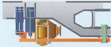
Front axle with three-point suspension and effective shock absorption.
