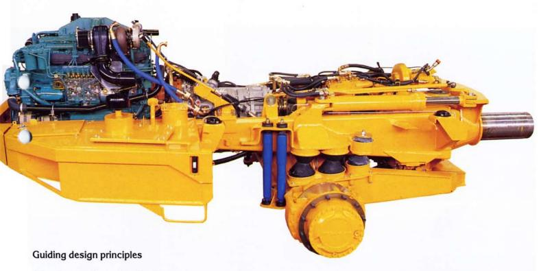
A fundamental principle for the terrainnegotiating capabilities of Volvo BM Articulated Haulers is the frame joint, which permits 360° rotation between the trailer and tractor units.
