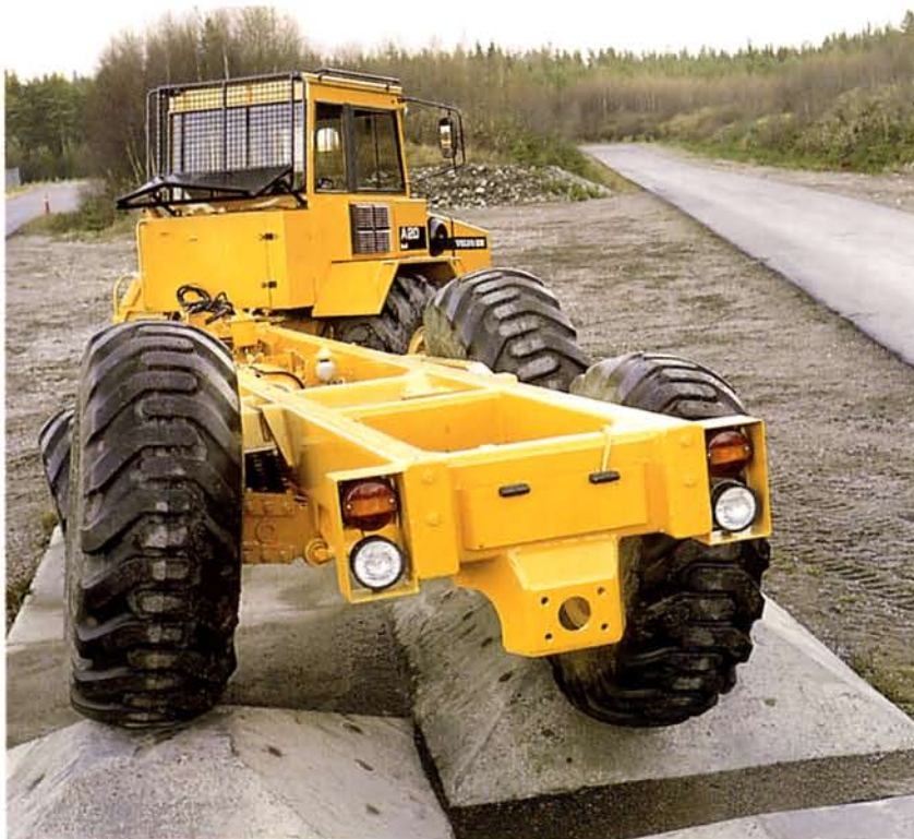
Volvo BM unique terrain bogie system with independent axle suspension, which can manage high obstacles without body movement.
