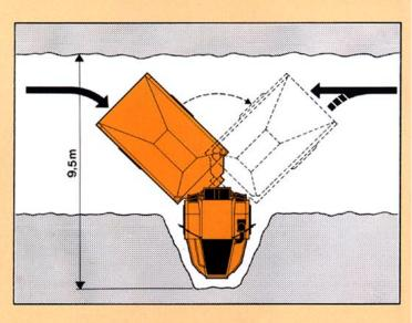
The turnaround system enables the A25B 4x4 to turn 180° easily in a width of only 9,5 m (31 ft).
