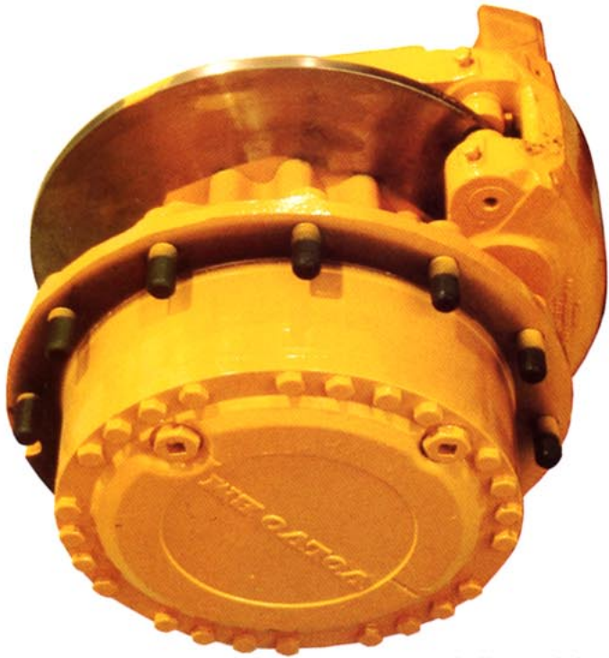
Well dimensioned all-round disc brakes ensure reliable performance under continuous repeated braking.
