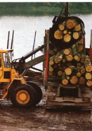
linkage system provides usually good breakout force even with the loader unit at top position.
