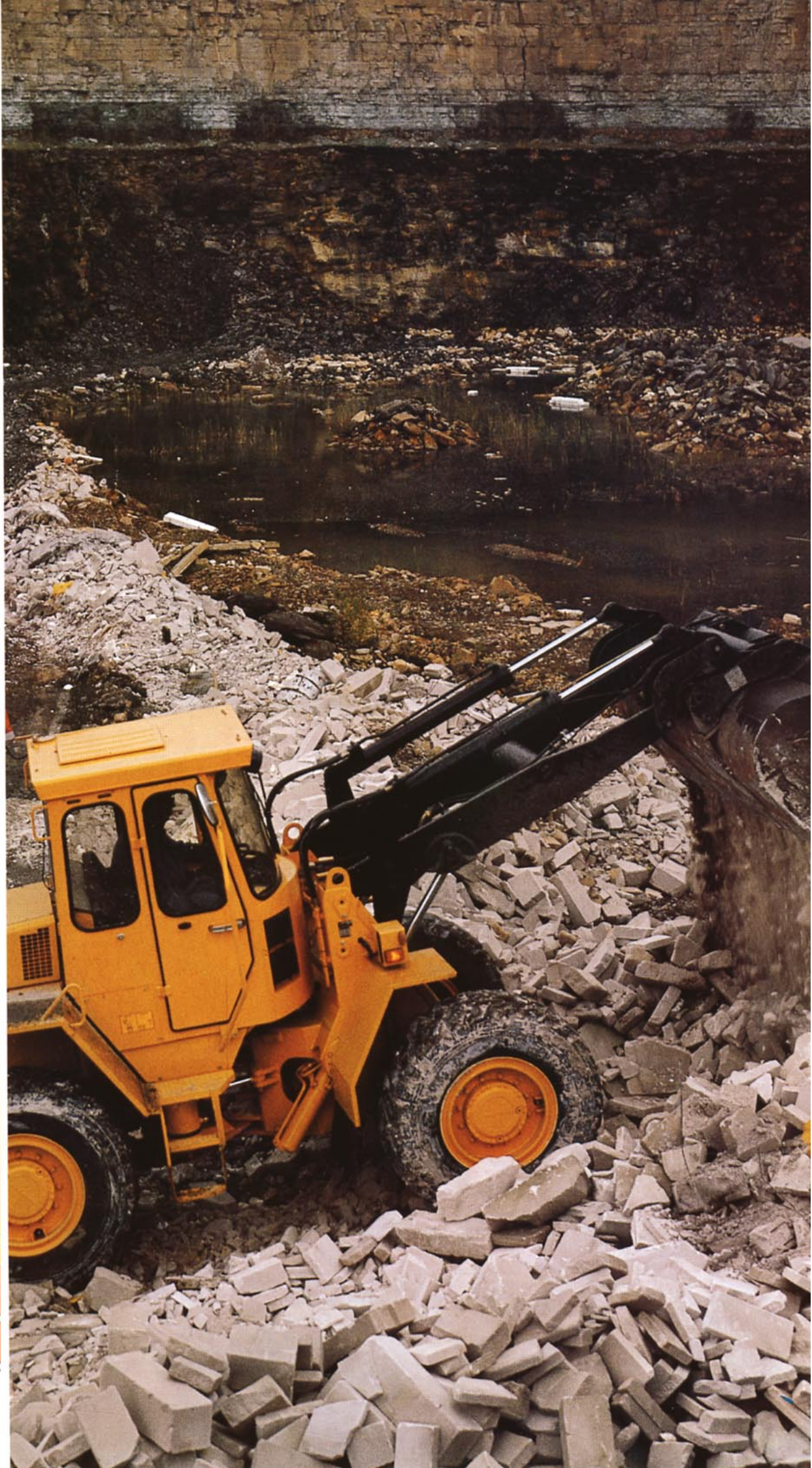
linkage system provides usually good breakout force even with the loader unit at top position.
