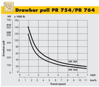
Usable drawbar pull will depend on traction and weight of tractor
