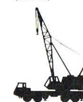
Wheel-mounted lattice boom cranes up to 165 tons (149.7 mt)
