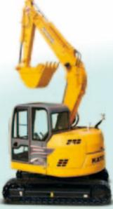
Improved Stability Increased tail radius and new shaped counter weight improve stability. Tail Slewing Radius: 1290mm (With Optional Weight): 1370mm
