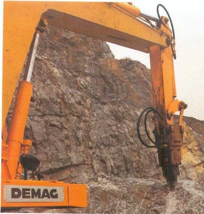
Demag Hydraulic Excavator with rock breaker; makes secondary blasting unnecessary.
