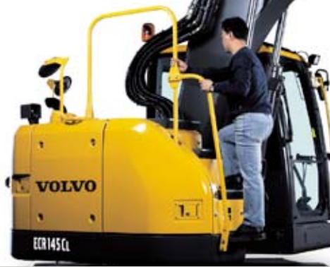
• 3-point, multi-purpose access with hand rail for ease and safety.
