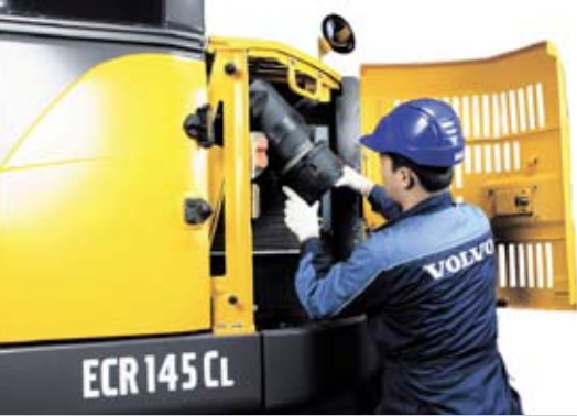
• Ground level air filter access.
