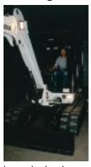
The standard lighting package includes both boom-mounted and frame-mounted adjustable lights. The frame-mounted unit is located on the left front corner of the machine. If additional lighting
