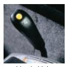
The two-speed activation function has been moved to the backfill blade handle. Pressing the two-speed button puts the
